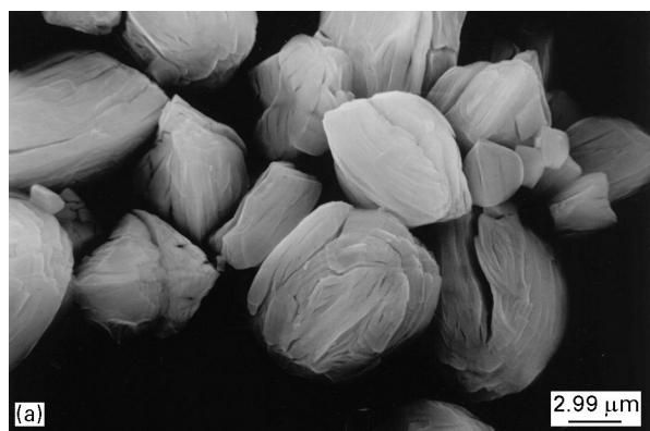
Figure 4 SEM images of nickel ferrite prepared at (a) 300 °C and (b) 495 °C.
